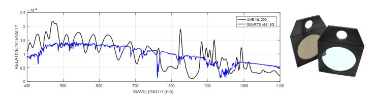
UHE-NL with AMF-AM1.5G filter installed providing class A spectral match to the AM1.5G spectrum
