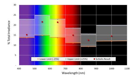
400-500 15.1774% Class A nm = 500-600 21.5593% Class A Class A 600-700 21.3764% Class A 700-800 14.9445% Class A 800-900 12.4609% nm = 900-1100 nm = 14.4815% Class A
